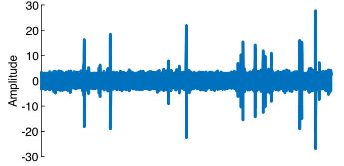
Fig. 5. Time domain waveform of recorded underwater ambient noise.
