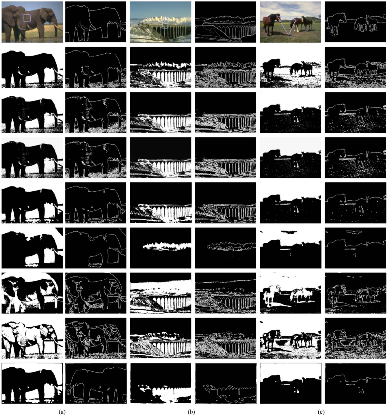
Fig. 6. Segmentation of real-world images. The first row presents the original images with the initial contour, and the corresponding human segmentation as ground truth. The second row presents the results of the proposed algorithm. The third row presents the results of the k -means clustering method. The fourth row presents the results of the FCM clustering method. The fifth row presents the results of the PKGC method. The sixth row presents the results of the CV method. The seventh row presents the results of the HZ method. The eighth row presents the results of the LI method. The last row presents the results of the GF method. For all the methods, the results are presented in two ways, i.e., by contours and binary images.
